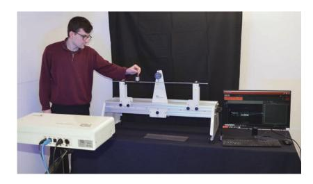
DefleX® is a contactless digital technique to help students learn how to measure and analyse deformations of objects optically. It is equipped with camera measurement and image processing software for analyzing motions, displacements and strains. It can measure visible features on objects and material surfaces like screws, joints, edges, grooves and composite structures.
