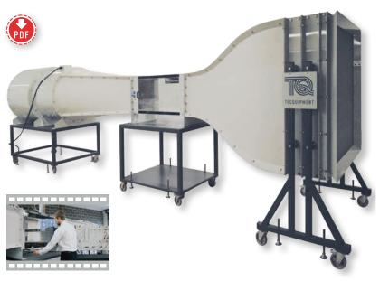
Larger open-circuit, suction subsonic wind tunnels for the study of advanced aerodynamics theory and research. With a working section of 450 mm or 600 mm comes greater visualisation and more accurate results, operating at meaningful Reynolds numbers.
