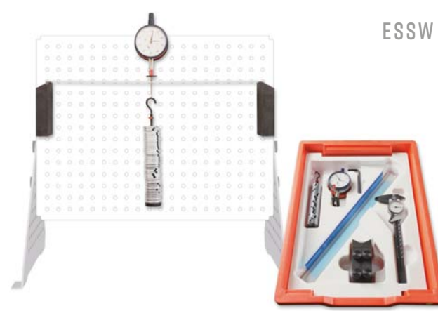
DEFLECTION OF BEAMS AND CANTILEVERS ES4
